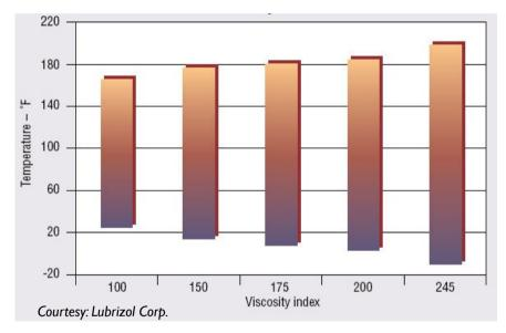
Figure B: Operating temperature ranges for ISO VG hydraulic fluid.
