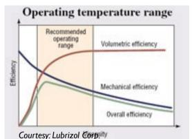
Figure D: Operating within the recommended viscosity range helps ensure that equipment is protected and that it operates most effi-
