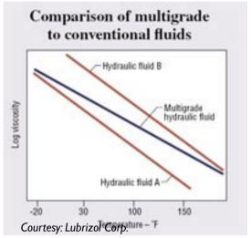
Figure C: Viscosity index for multigrade fluids shows how they offer both low-temperature fluidity and high-temperature viscosity.
